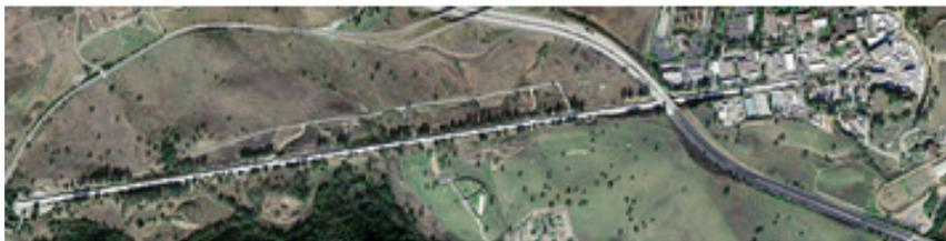
Aerial photo of the Stanford Linear Accelerator Center, with detector complex at the right (east) side
